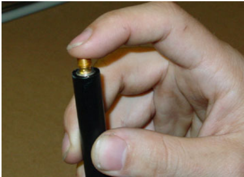
Figure 17. Centering antenna in radome while epoxy sets.
