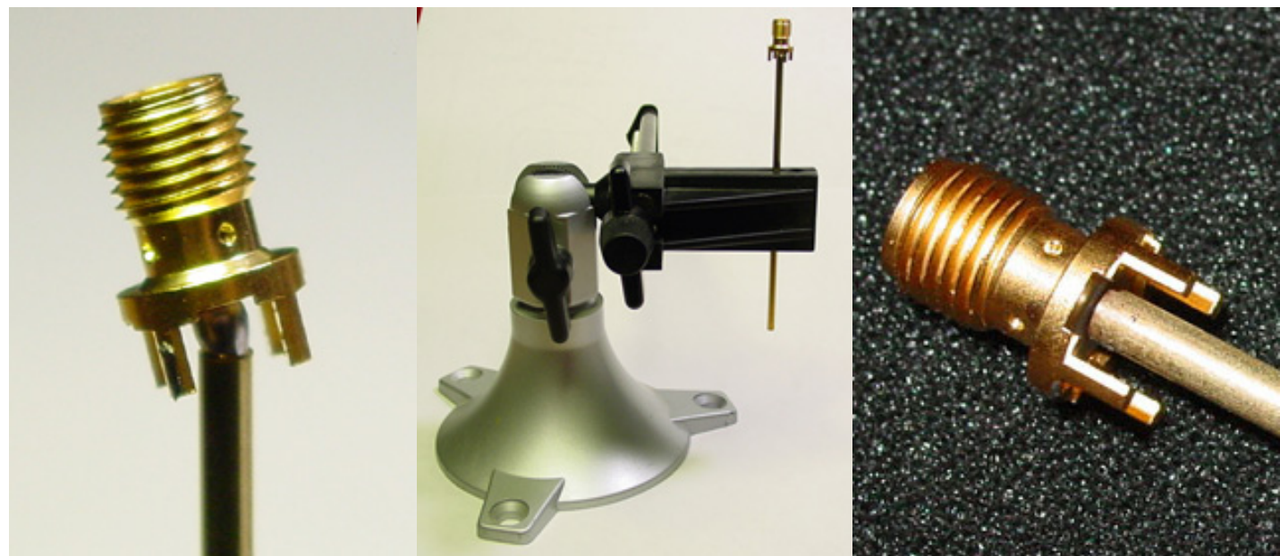
Figure 5: The image on the left shows the solder applied to the center conductor now resting on the feed prior to feedline heating. The center image shows the feedline in vise, after heating the tube and allowing the connector to rest flat on the top of the feedline tube. The image on the right shows the completed feedline soldered to SMA center conductor.
