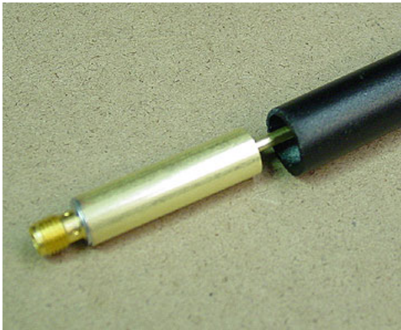
Figure 14. Leave enough room to apply epoxy into the decoupler end of the radome.
