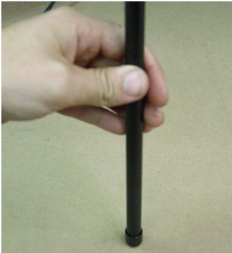
Figure 19. Holding the antenna on the cap until epoxy cures.
