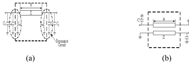
Fig. 1 Hirota's reduced size \lambda/4 line including artificial resonance circuit (a) and the equivalent coupled lines circuit (b).
