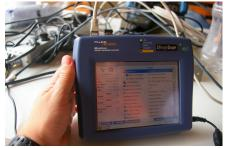
The test uses different packet sizes (64, 128, 256, 512, 1024, 1280, 1518) and applies the same load for each of these. We used 99,99% measurement accuracy for the testing which means that the Fluke units measured the dropped or retransmitted packets and decreased the load until the link reached 99,99% availability which means the pure and accurate throughput of the radio links.
