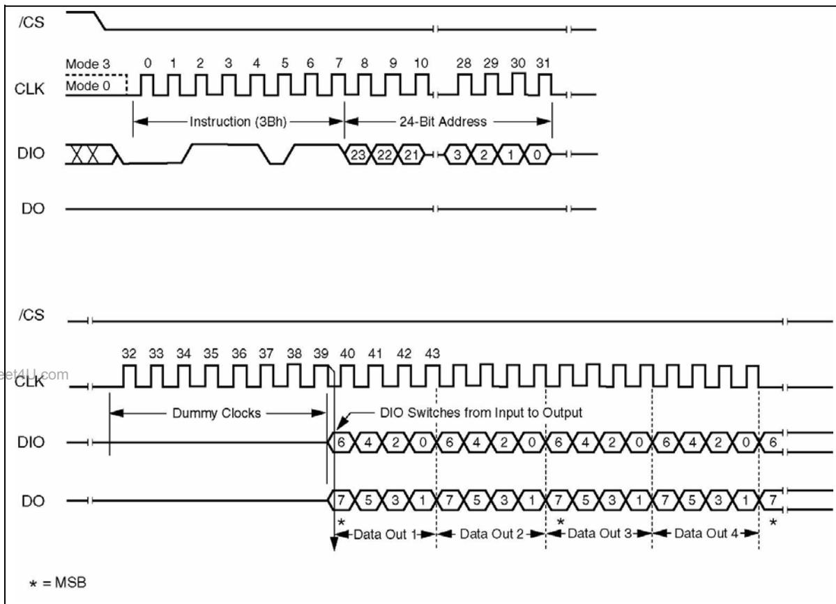
Figure 10. Fast Read Dual Output Instruction Sequence Diagram
