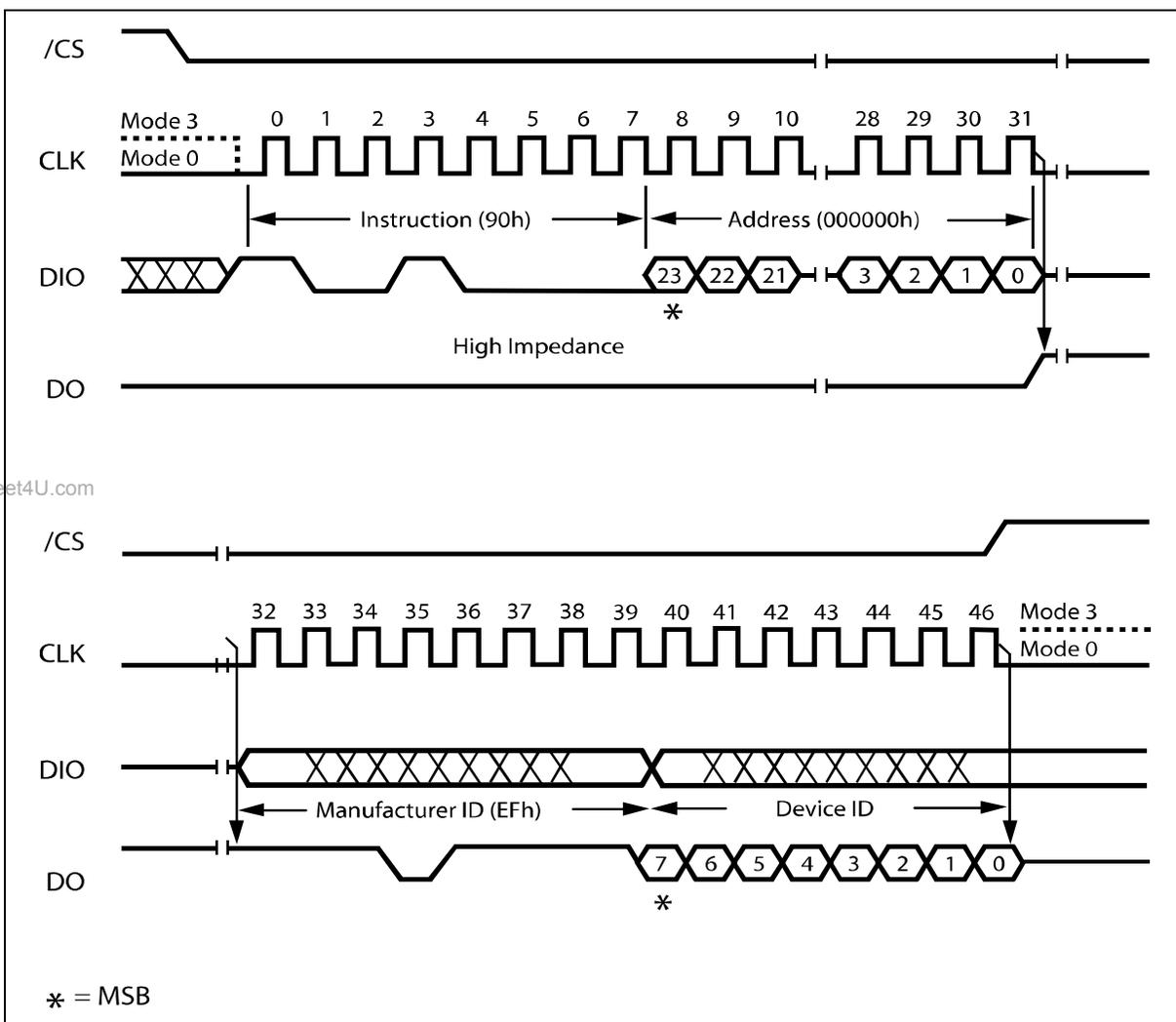
Figure 18. Read Manufacturer / Device ID Diagram
