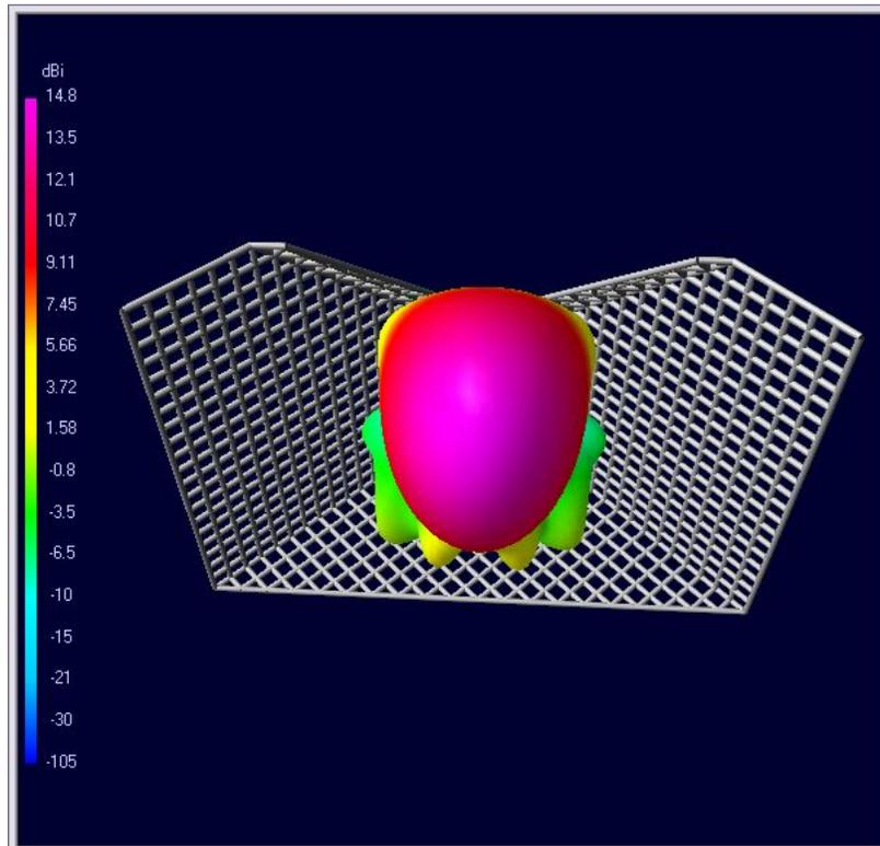
**Fig. 9. Main beam of Truncated 3D Corner Reflector Feed**
