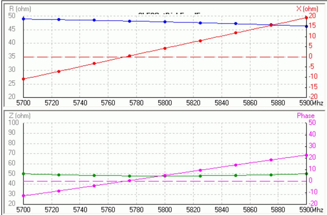
**Fig. 8. Input impedance of Truncated 3D Corner Reflector Feed**
