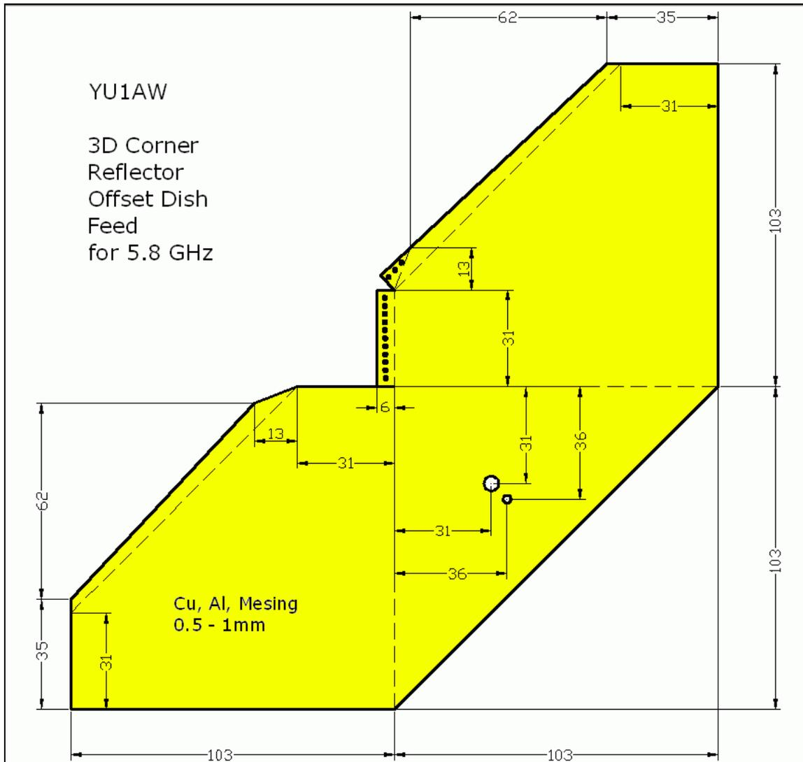
**Fig. 13. Cut dimensions and bending lines for reflector of Truncated 3D Corner Reflector Feed**
