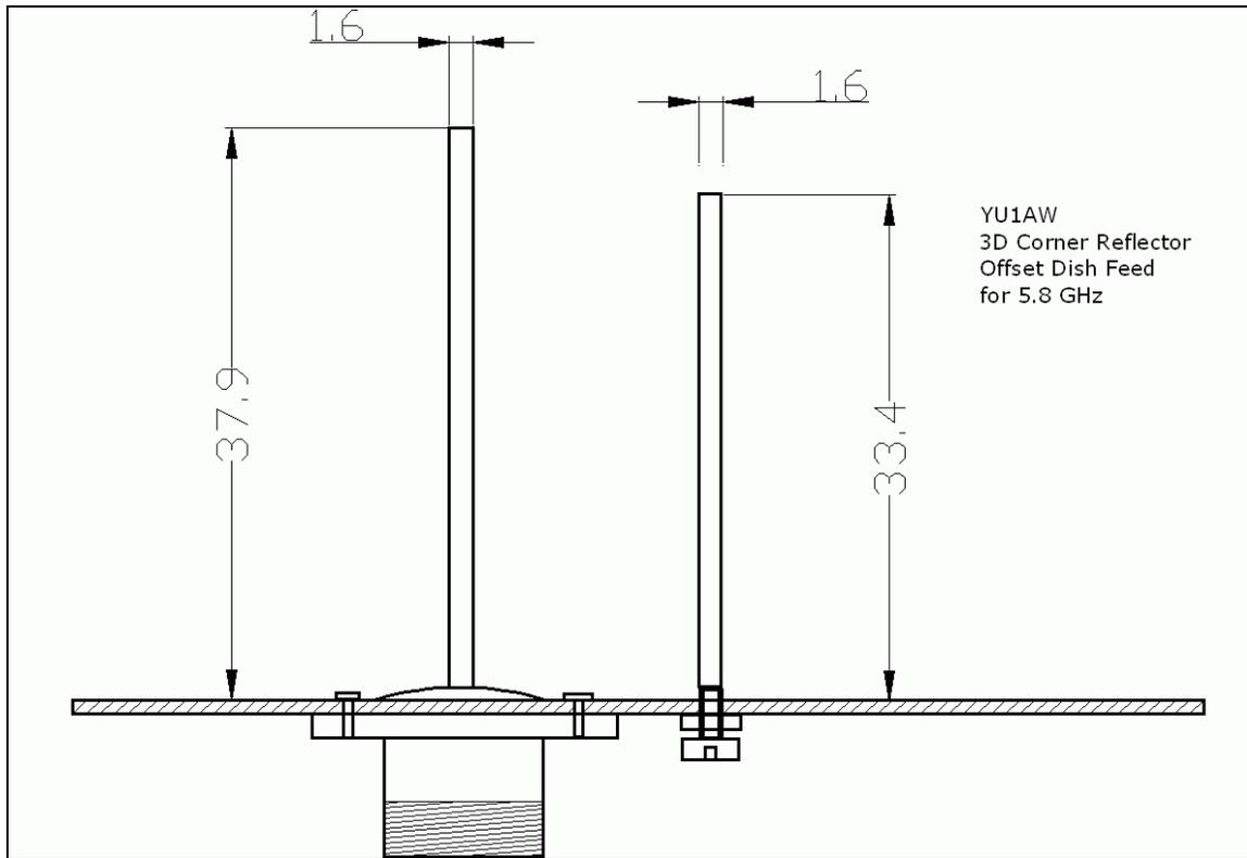
**Fig. 14. Elements dimension of Truncated 3D Corner Reflector Feed**
