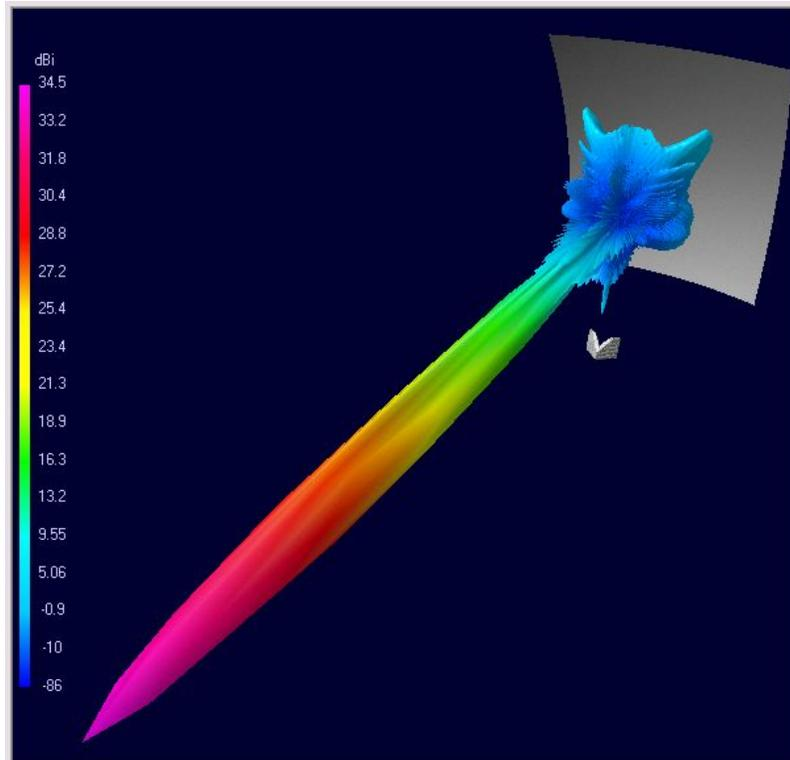
**Fig. 18. 3D diagram of rectangular offset parabola with Truncated 3D Corner Reflector Feed**
