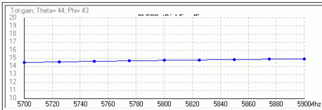
**Fig. 5. Truncated 3D Corner Reflector Feed gain**
