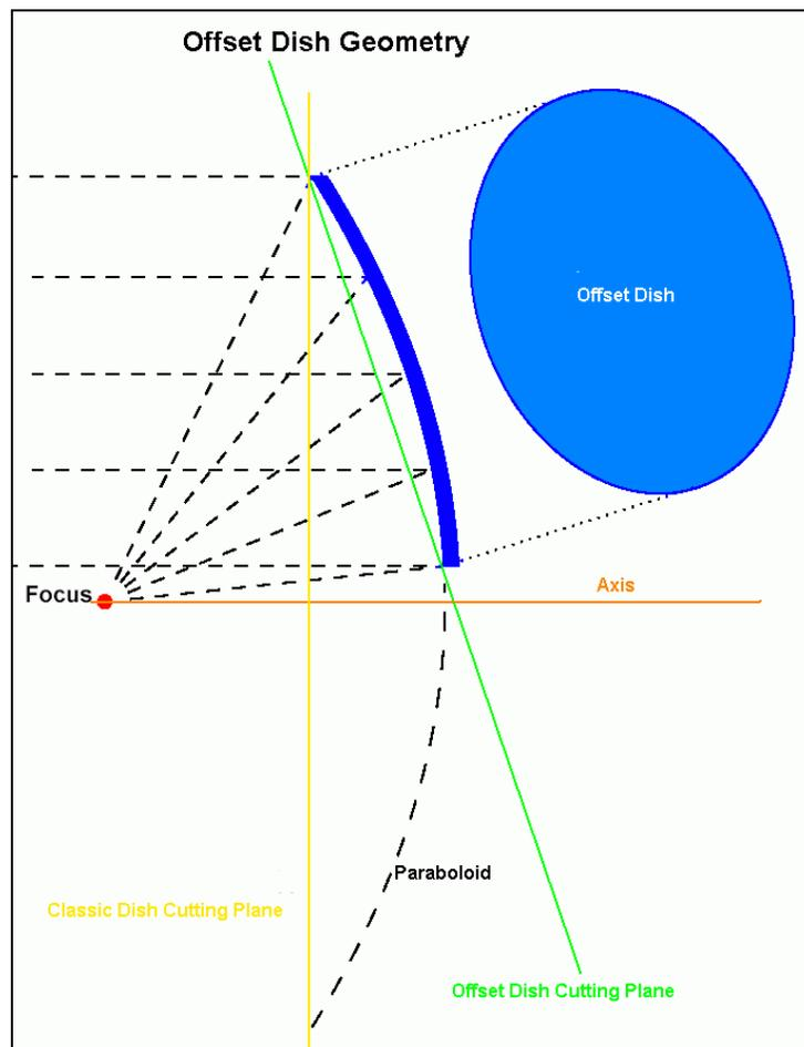
**Fig. 1. Offset parabola geometry**
