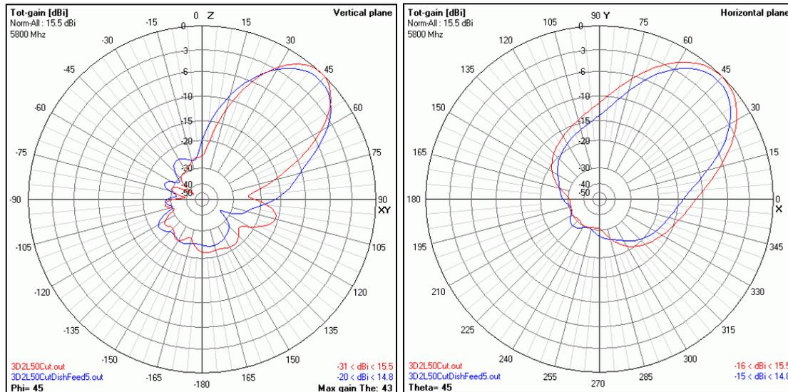
**Fig. 4. Comparative diagrams for shortened 3D corner reflector antenna of 2 wavelengths and truncated 3D corner reflector feed**
