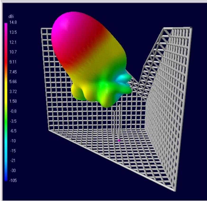
**Fig. 6. 3D radiation diagram of Truncated 3D Corner Reflector Feed**
