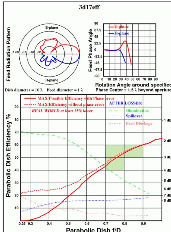
**Fig. 3. Offset parabola efficiency with 3D corner reflector antenna of 1.7 wavelength feed at 5.8 GHz frequency.**
