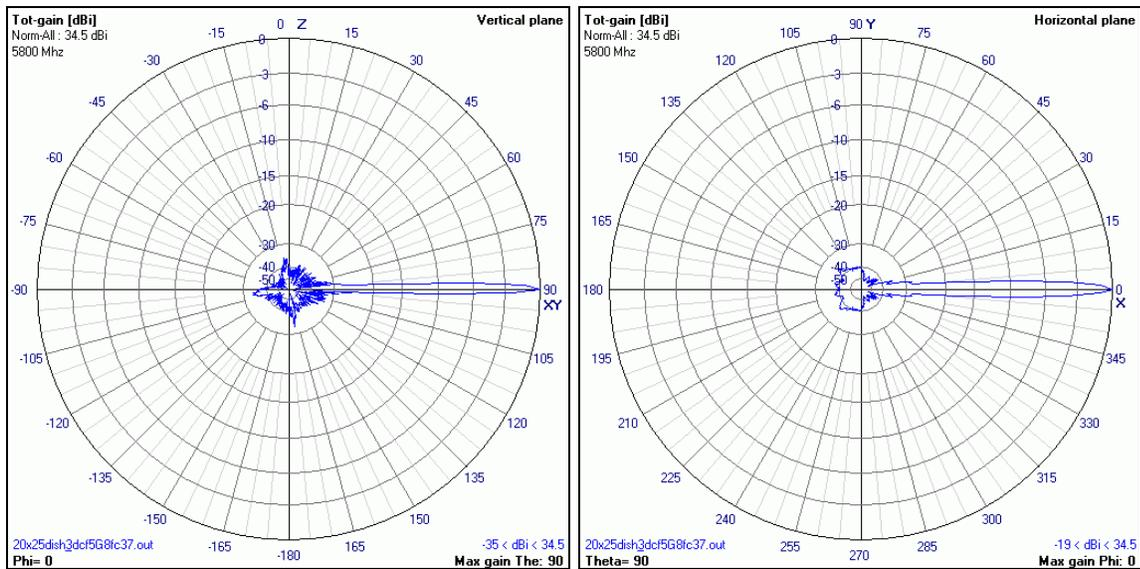
**Fig. 16. Vertical and horizontal diagrams of offset parabola with Truncated 3D Corner Reflector Feed**
