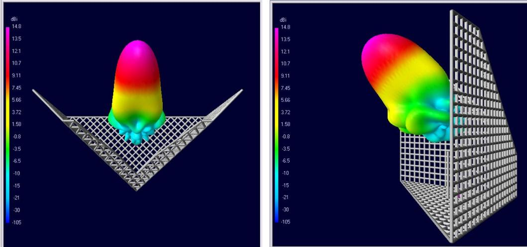
*Fig. 10. Horizontal and vertical diagram of Truncated 3D Corner Reflector Feed*
