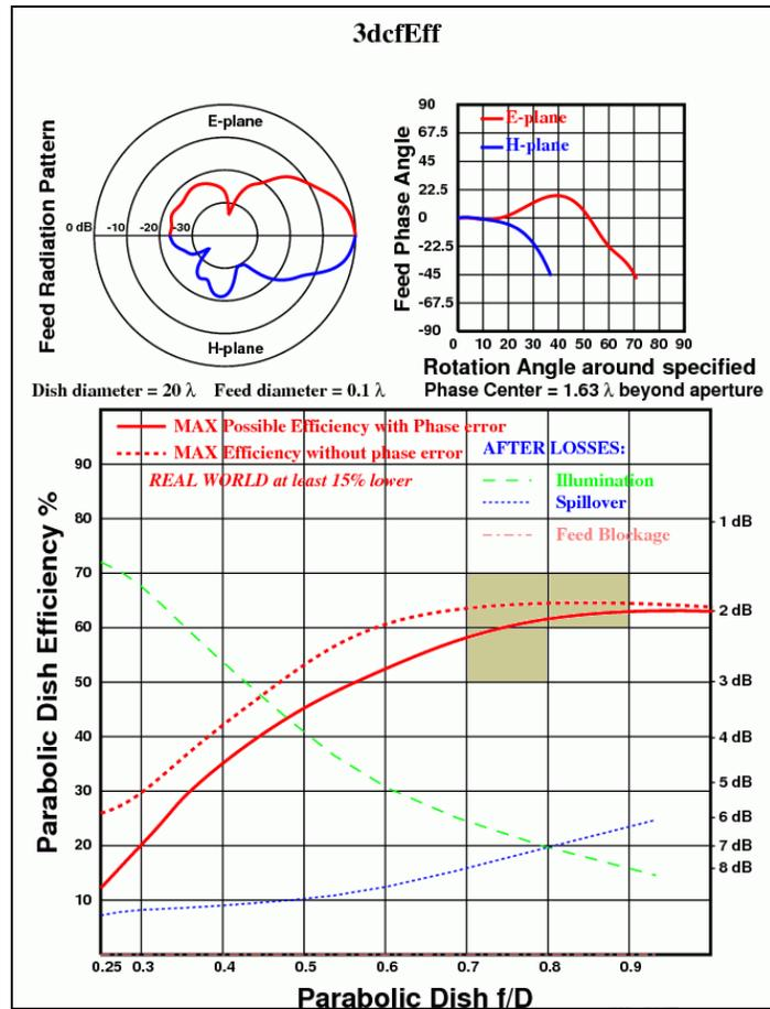
**Fig. 17. Parabola efficiency with Truncated 3D Corner Reflector Feed in relation to its F/D ratio**
