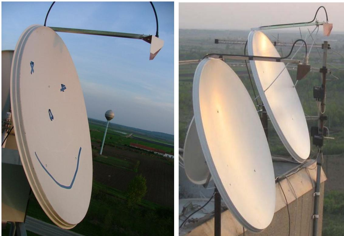
**Fig. 21. 50 km 5.8 GHz link using offset parabola dish and Truncated 3D Corner Reflector Feed**
